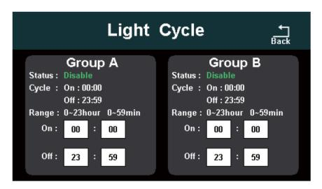
IN Auto mode, set turn on time and turn off time, timing cycle is 24 hours.
