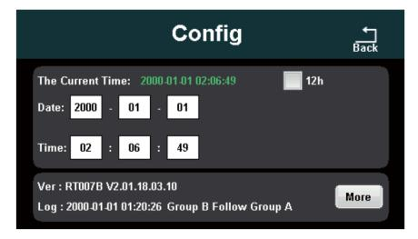
Work Log: You can review work log when press "More" Time setting: the default is 24 hours time system; when click "12h", it will enter into 12 hours time system.
